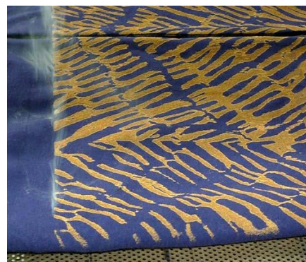
Figure 6 - Laser engraved wool/polyester fabric with graphic method
