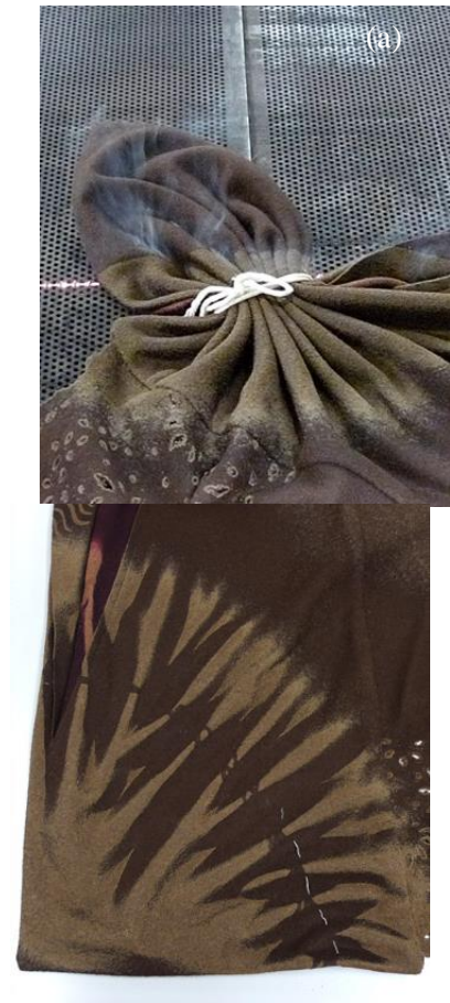
Figure 7 - Laser engraved wool/polyester fabric with resist method
